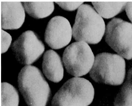
Figure 2 —Microencapsulated beads; calculated film thickness = 6.6 \mu\text{m} .
