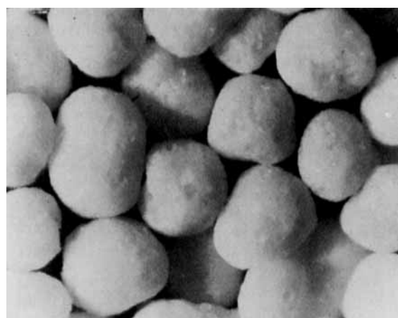
Figure 1 —Marumerized cores prior to microencapsulation containing 12.08% bitolterol mesylate; mean volume-surface diameter = 784 μm.
